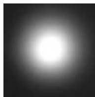
NAPL-3DIFF Diffused Lens with 26° TIR Optic
